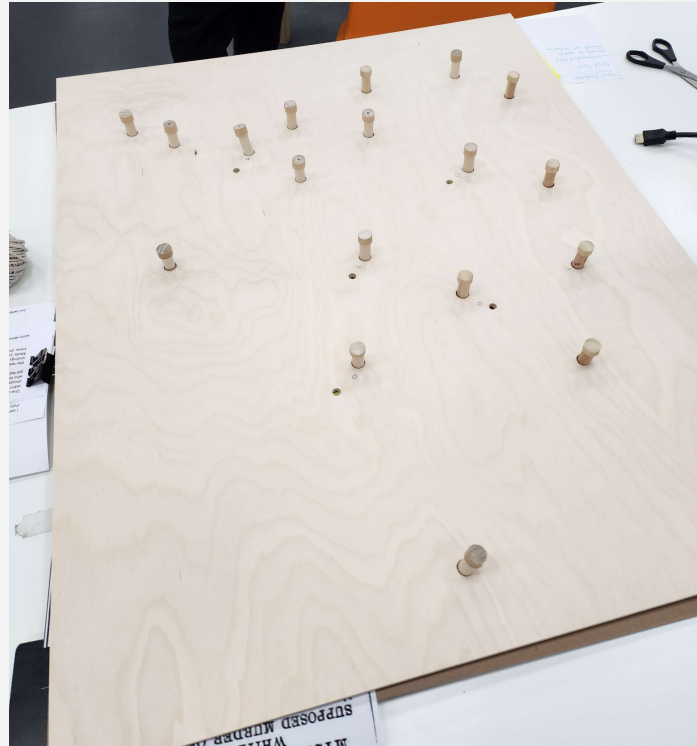
Figure 65: Board after cut and drills with wooden pegs
